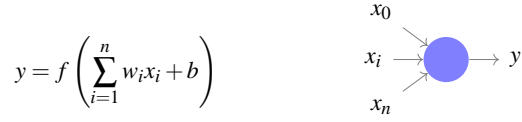
FIG. 7. Schematic and mathematical representation of a neuron. A neuron takes multiple inputs, multiplies each input with a weight w_i , sums the results, adds a bias b and applies an activation function f . Generally f is a nonlinear function.
