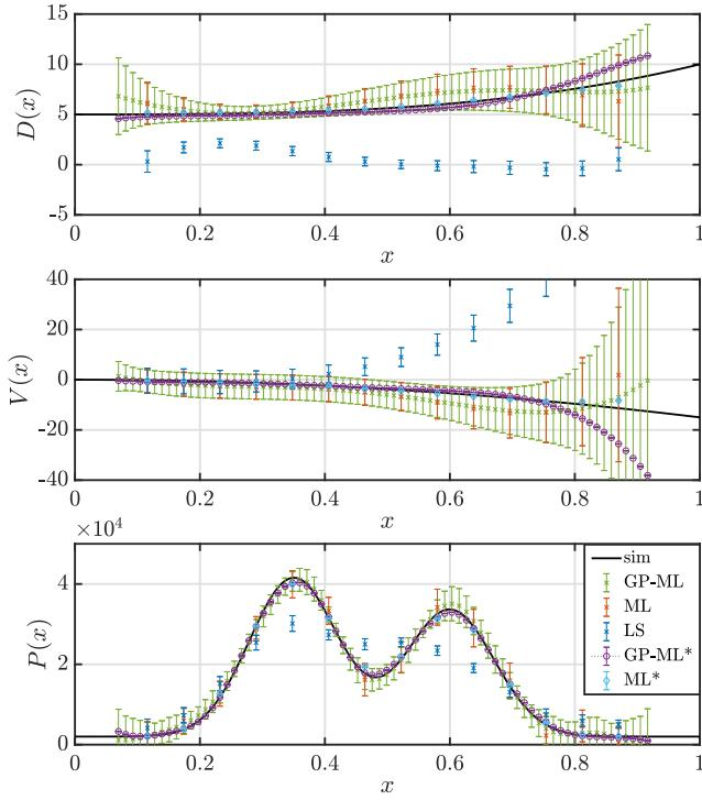
Fig. 2. The estimated transport parameters: diffusion (top), convection (middle), source location (bottom) and their  $p = 0.95$  confidence interval, estimated by the earlier presented ordinary least squares method (LS), the novel maximum likelihood method (ML) and the maximum likelihood method where the state and its uncertainty is estimated using Gaussian process regression (GP-ML) where the \* indicates the noiseless scenario.
