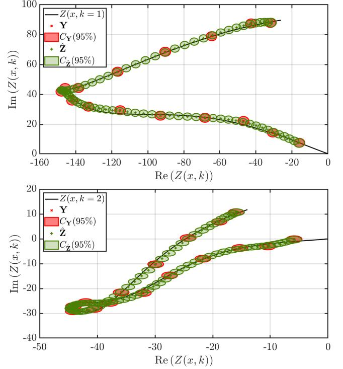
Fig. 1. The simulated  $Z$ , measured  $\mathbf{Y}$  and estimated state  $\hat{Z}$  shown in the complex plane for the first harmonic ( $k = 1$ ) at  $\omega = 50$  (top) and the second harmonic ( $k = 2$ ) at  $\omega = 100$  (bottom), including their  $p = 0.95$  confidence interval.
