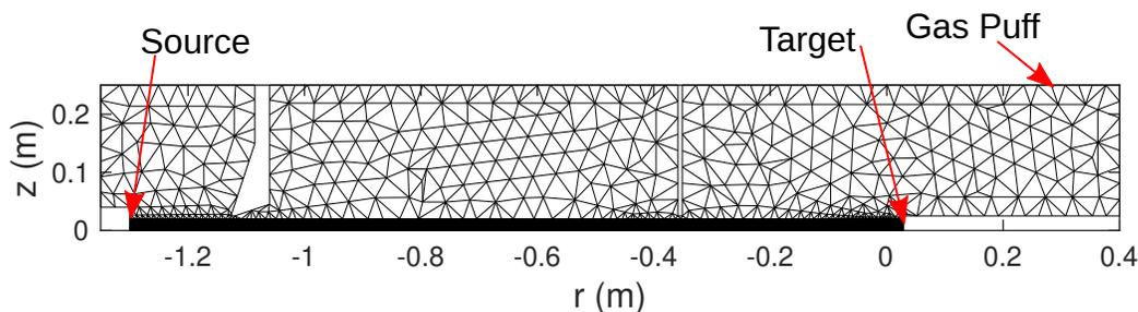
Figure 2: Eirene mesh used for the high density case in this work. The dark region at the axis represents the plasma grid. The Eunomia mesh and the meshes used for the low density case are qualitatively similar and are not shown here for the sake of simplicity.
