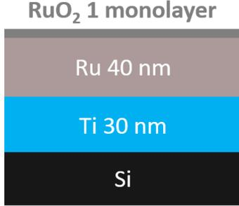
Figure 1: Schematic of the film stack of the target before Sn deposition.
