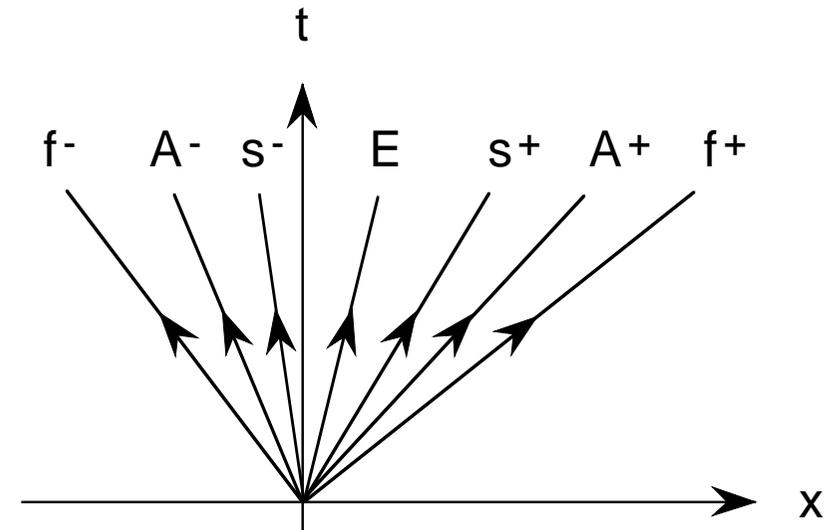
Group diagram is the *ray surface*, i.e. the spatial part of characteristic manifold at certain time  $t_0$ .
