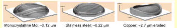
Fig. 17. Erosion of three different materials after long time exposure to the Tore Supra plasma. The effects on the reflectivity were only small.
